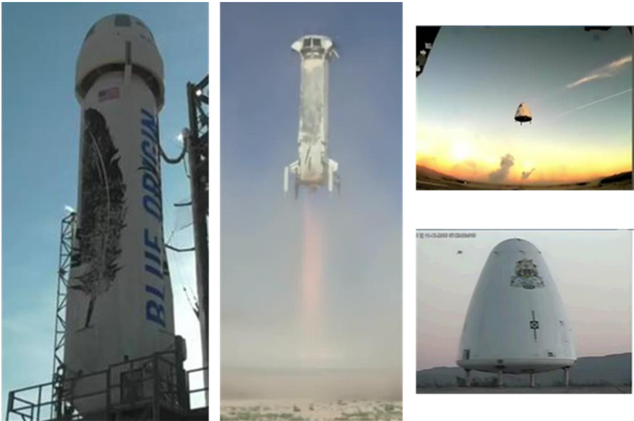
Figure 2.5. Field tests of landing systems of elements of the space launch vehicle and piloted vehicle carried out by Blue Origin Blue Origin's illustrations
