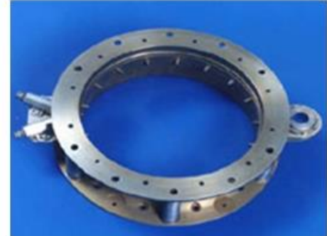
Figure 7.4 Typical devices for SC separation from the launch vehicle (clamping band-type adapter scheme and explosive ring adapter for microsatellites)
